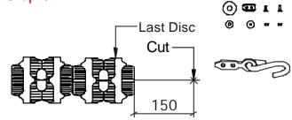
Cut the Stainless Steel Cable as above drawing, then uninstall the Long Clamp.
